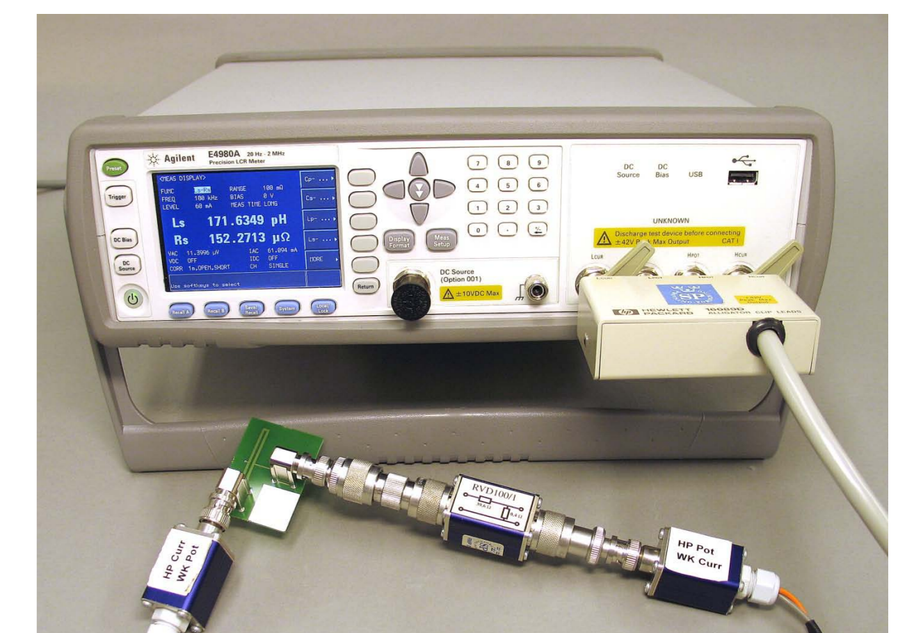
Figure 3 Test of method by measurements with "known" standards.
